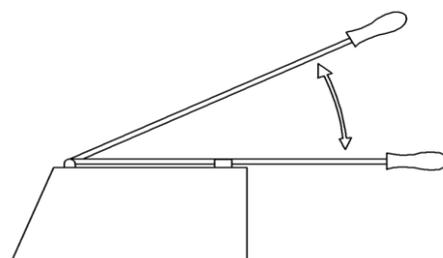
Release and move forward the handle of the scoop to remove it. Discard the contents on the ash deposit.
