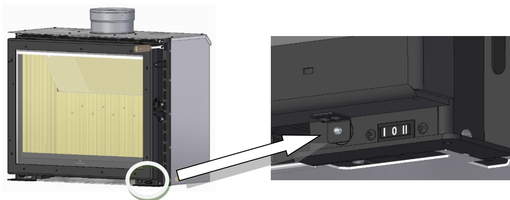
Figure 51 – Door handle adjustment, micro-switch actuation
