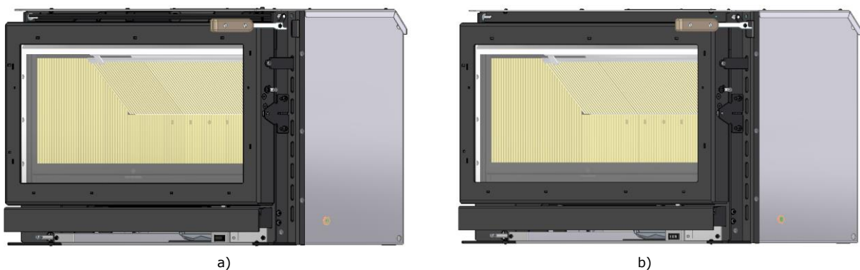
Figure 23 - a) Fan warm air control mechanism Open, b) Fan warm air control mechanism Closed
