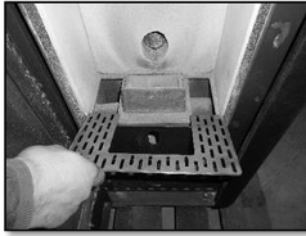
Figure 15 - Removing the ash pan grate
