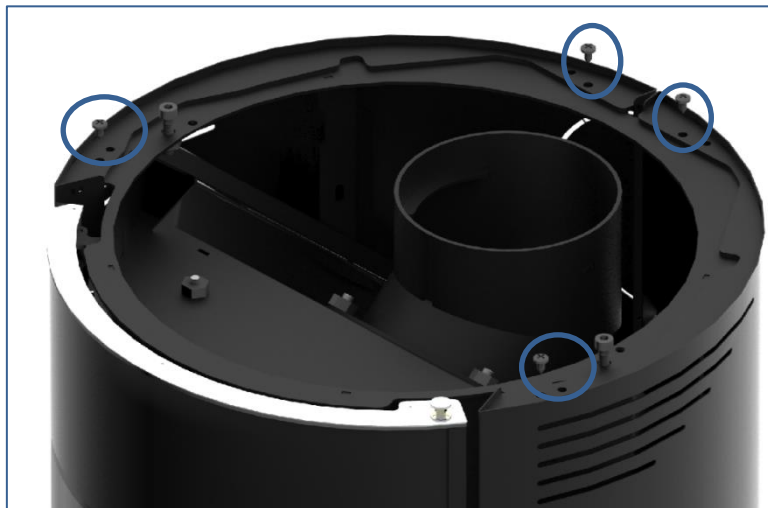
Figure 17 – Disassembly of the side casings in the equipment
