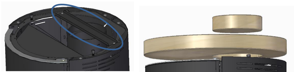
Figure 15 – Placing the top cover on the equipment with horizontal smoke outlet
