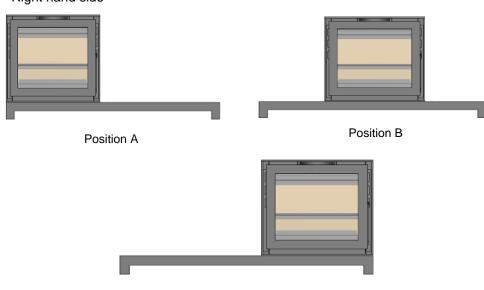
To mount the base, set it on the desired location and then place the unit in the selected position. Place the free standing fire unit on the supporting base, carefully matching the screw holes on the bottom relative to the intended position (K and L) with the guide pins (J) on the supporting base.
