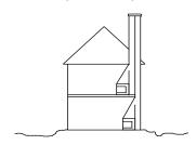
• The flue must be free from obstructions, and preferably maintain the same round diameter all the way through, from the unit to the output. To ensure proper operation, the diameter must be compliant with each model specifications (refer to the catalogue).
